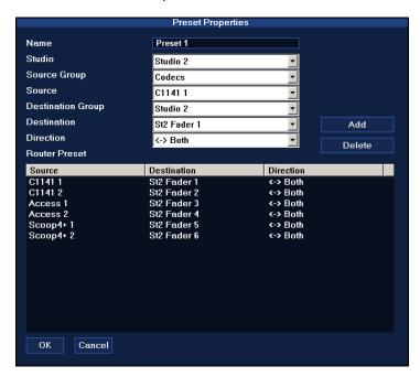
A very powerfull option within the MDC.net routing system is the ability to store routing presets. The presets allow multiple crosspoints to be set or cleared with just a single mouse-click. A preview window shows the crosspoints to be made (or cleared) prior to the actual routing.
